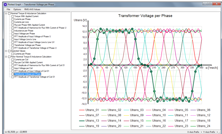
Abb. 225: Universal Motor - Transformer Voltage per Rotor Phase (Rotor Current = 0A)
